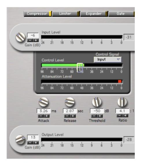
Any more than 6dB of compression will start to be noticeable. Poorly compressed signals will sound like pumping or breathing, and background noise becomes apparent.
